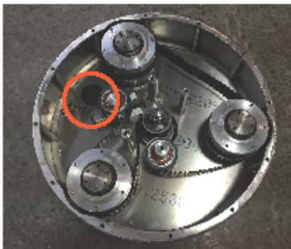
Fig 3. Plastic cap for removal. (Bottom plate removed for easier identification.)
